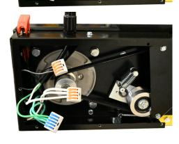
The light has its own rotary switch on the lamp shade. This way you can use the light even if the sharpener isn't running.
